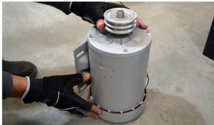
Fig.39 - Polia instalada no motor
