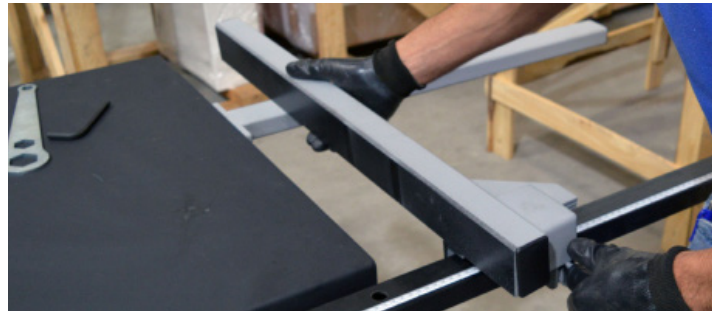
Fig.25 - Guia Exakta instalada
